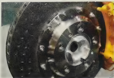
A ceramic brake disc in a sports car withstands temperature of 1400 °C.
