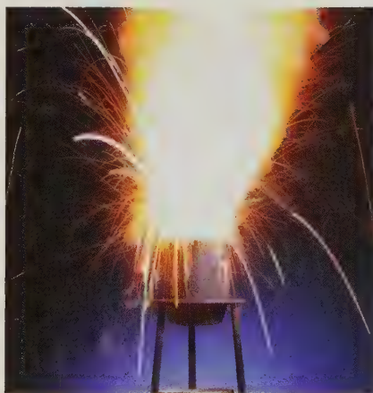
Aluminum and iron(III) oxide produce heat in an exothermic reaction.
