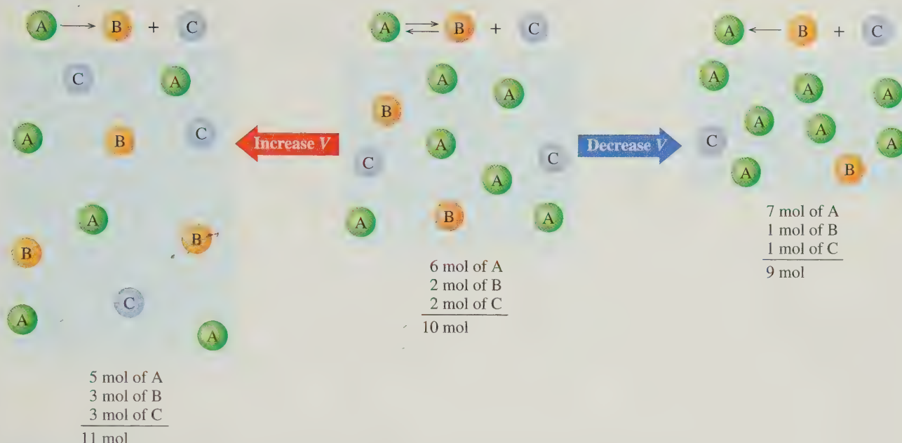
FIGURE 13.13 The decrease in the volume of the container places stress on the equilibrium \text{A(g)} \rightleftharpoons \text{B(g)} + \text{C(g)} . To relieve the stress, the reverse reaction converts some products to reactant, which gives a smaller number of moles of gas, reduces pressure, and reestablishes the equilibrium. When the volume increases, the forward reaction converts reactant to products, which increases the moles of gas and relieves the stress.
