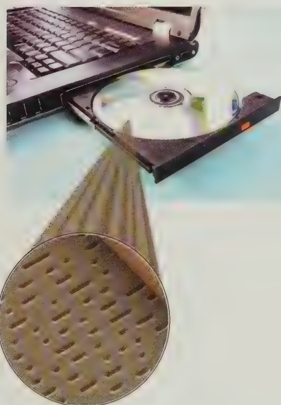
A CD or DVD is read when light from a laser is reflected from the pits on the surface.
