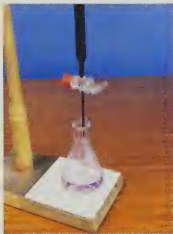
In an oxidation-reduction titration, the \text{KMnO}_4 in the buret reacts with \text{Na}_2\text{C}_2\text{O}_4 .
