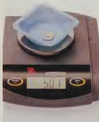
FIGURE 2.3 On an electronic balance, a nickel has a mass of 5.01 g in the digital readout.
